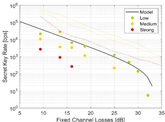
Effect of atmospheric turbulence on satellite QKD channel losses.
