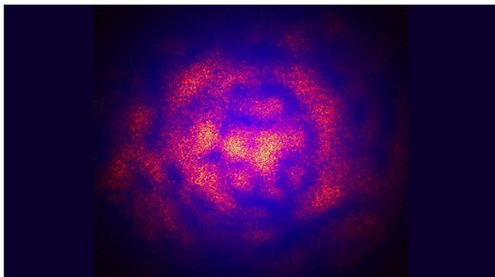
*A laboratory image showing a chaotic speckle pattern that results from quantum particles of light being scrambled by a complex medium such as a multi-mode optical fibre.*
