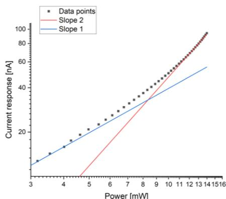
Fig 1. The current response of a silicon photodiode as the incident power is increased. The TPA data is displayed as a log-log plot, where the blue line is of slope 1, indicating SPA, and the red line has a slope of 2 representing TPA.
