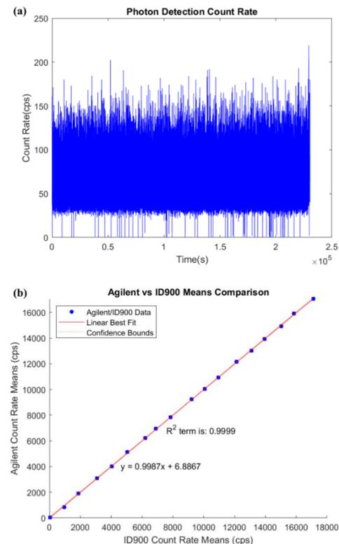
Fig 3 (a). The resulting output count rate over 64 hours of the Agilent using the Matlab code. (b) Linear regression comparison plot of Agilent data vs ID900 data from a dark count rate to ~18kc/s in 1kc/s steps as best as the lighting conditions could be restricted.
