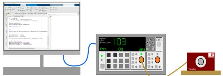
Fig 1. Diagrammatic set-up used to record data using the photon detector. To record a dark count, a blackout sheet was also used to cover the detector.
