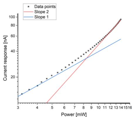
Fig 1. The current response of a silicon photodiode as the incident power is increased. The TPA data is displayed as a log-log plot, where the blue line is of slope 1, indicating SPA, and the red line has a slope of 2 representing TPA.
