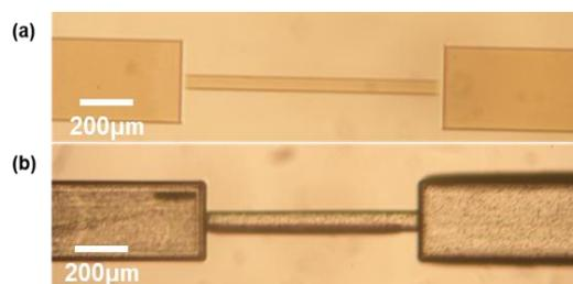
Fig 1. Images of 50 $\mu\text{m}$  wide microfluidic channel with 300 $\mu\text{m}$  wide inlet and outlet, written at 2mm/s at 340mW with horizontal polarisation (a) before etching in KOH and (b) after etching in KOH.
