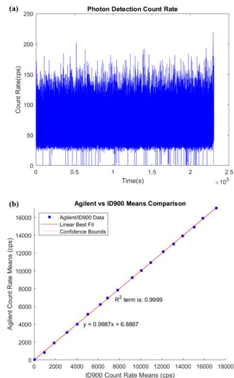
Fig 3 (a). The resulting output count rate over 64 hours of the Agilent using the Matlab code. (b) Linear regression comparison plot of Agilent data vs ID900 data from a dark count rate to ~18kc/s in 1kc/s steps as best as the lighting conditions could be restricted.
