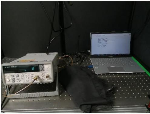
Fig 2. The actual set-up recording data in the lab. As you can see, the count rate is displayed on the frequency counter whilst the blackout sheet is covering the photon detector to record a dark count rate.
