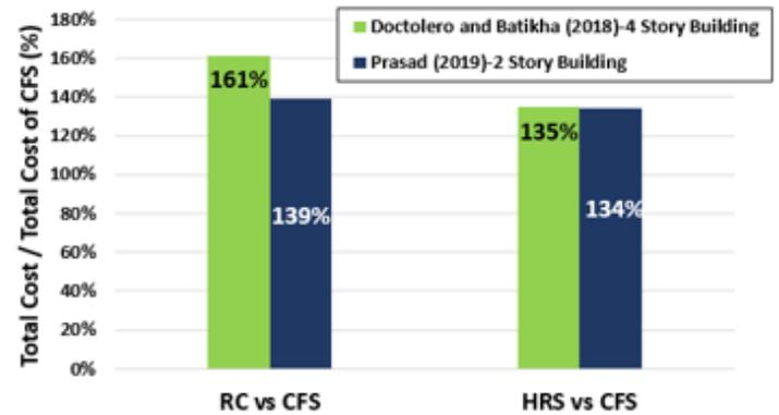
**Fig. 6.** CFS vs RC and HRS in terms of the total construction cost.
