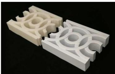
**Fig. 2.** Side-by-side comparison of a grill diffuser manufactured using traditional methods vs 3D printed methods.
