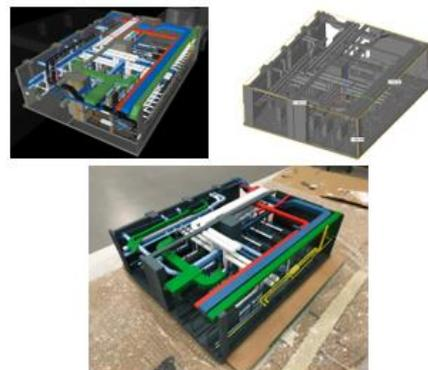
**Fig. 1.** BIM model vs digital 3D printing model and the final 3D printed product.
