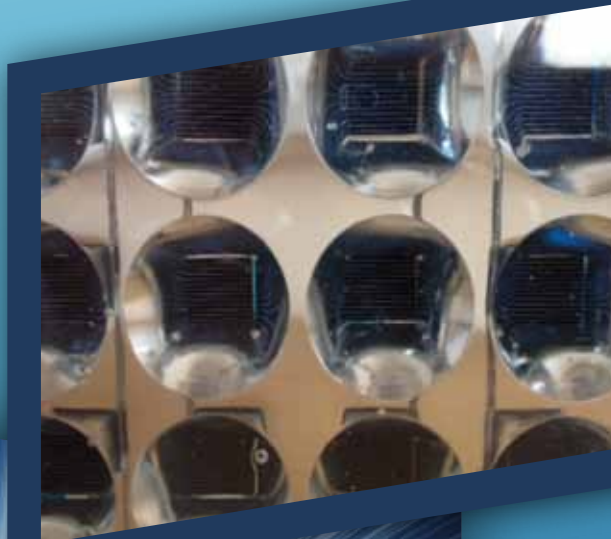
Figure 1: The prototype non-imaging concentrator design has a wide acceptance angle of 120^\circ ( -60^\circ to +60^\circ ) to maximise the sunlight captured between dawn till dusk and a range of concentration factors (1x to >10x ) is available depending on the performance needs.
