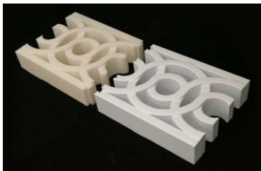
Fig. 2. Side-by-side comparison of a grill diffuser manufactured using traditional methods vs 3D printed methods.
